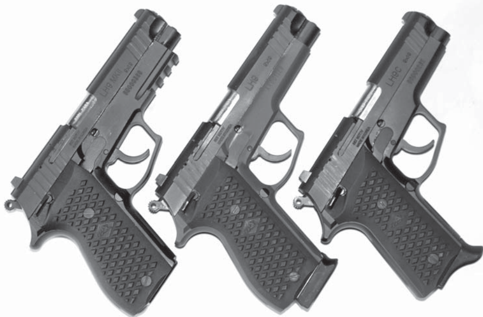
Below: Lion-Heart is a new company offering a 9mm pistol family with a unique firing system of DA/SA, SA cocked and locked, and hammer down semi-cocked. It is based on the FN-Fast Action pistol. A .40-caliber version is planned.
